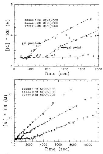
Figure 7 Radical concentration versus time for ST/UPE resins with MR=4 and various amounts of initiator cured at  $40^{\circ}C$
