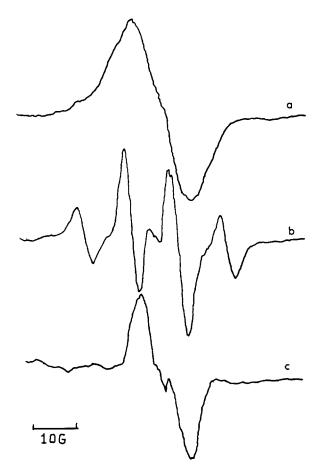
Figure 5 E.s.r. spectra of UPE in toluene with 1.0% MEKP/COB after 1 week (a); ST/UPE resin with MR=2 and 1.0% MEKP/COB at room temperature (b) and at  $-50^{\circ}$ C (c)
