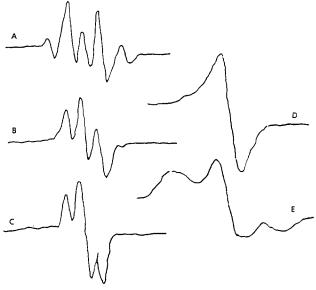
Figure 1 Typical e.s.r. spectra observed during the reaction of ST/UPE resins: A, induction period; B, reaction start; C, transition; D, macrogelation; E, cured
