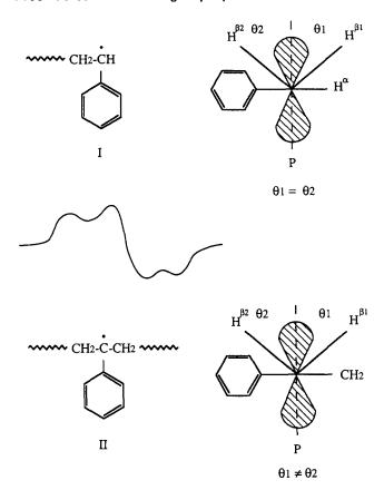
Figure 2 Chemical formula, radical structure and e.s.r. spectrum of ST-end stable radicals (P is polymer chain)
