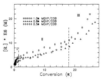
Figure 8 Radical concentration *versus* conversion for ST/UPE resins with MR=4 and various amounts of initiator cured at 40°C
