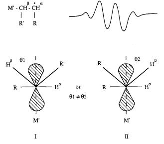
Figure 3 Chemical formula, radical structure and e.s.r. spectrum of UPE-end growing radicals (R and R' are repeating unit of UPE chain and M' is oligomer formed through chain reaction)
