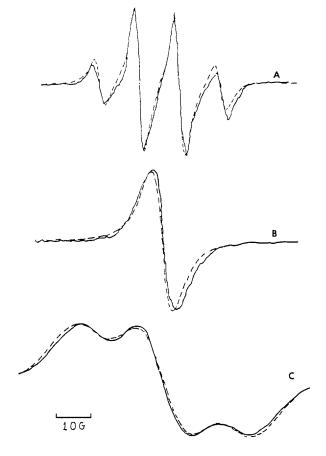
Figure 6 Comparison of simulated (---) and measured (---) e.s.r. spectra of various radicals: A, UPE-end growing radical; B, UPE-end stable radical; C. ST-end stable radical
