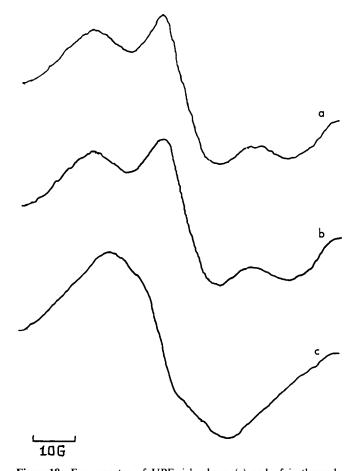
Figure 18 E.s.r. spectra of UPE-rich phase: (a) end of isothermal reaction at  $40^{\circ}$ C; (b) end of temperature scanning run at  $113^{\circ}$ C; (c) after 3 h of post-cure at  $140^{\circ}$ C
