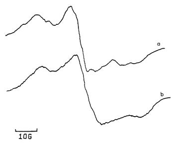
Figure 15 E.s.r. spectra of the 30°C isothermally cured ST/UPE resin with MR=4: (a) end of curing; (b) after storage for 1 month
