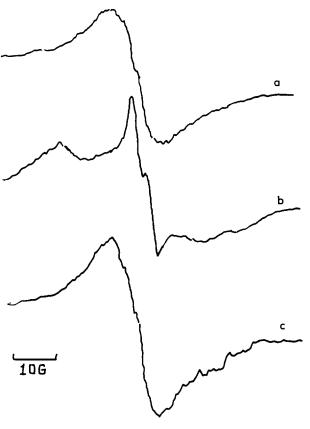
Figure 19 E.s.r. spectra of ST-rich phase: (a) end of isothermal reaction at 40°C; (b) end of temperature scanning run at 113°C; (c) after 3 h of post-cure at 140°C
