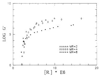
Figure 11 Shear storage modulus versus radical concentration for ST/UPE resin with 1.0% MEKP/COB cured at 40°C with various values of MR
