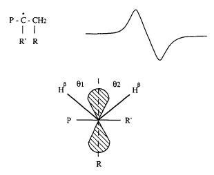
Figure 4 Chemical formula, radical structure and e.s.r. spectrum of UPE-end stable radicals (R and R' are repeating unit of UPE chain and P is polymer chain)
