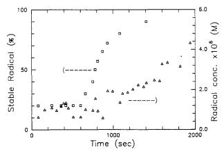
Figure 13 Stable radical percentage and radical concentration *versus* reaction time for ST/UPE resin with MR = 2 and 1.0% MEKP/COB cured at 40°C
