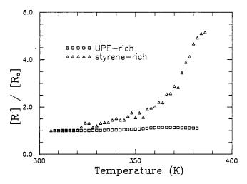
Figure 17 Relative radical concentration of temperature scanning reaction of 40°C isothermally cured ST-rich and UPE-rich samples
