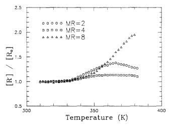
Figure 16 Relative radical concentration of temperature scanning reaction for 40°C isothermally cured ST/UPE resin with 1.0% MEKP/COB and various values of MR
