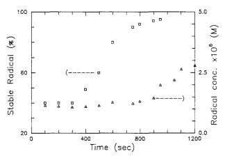
Figure 14 Stable radical percentage and radical concentration versus reaction time for ST/UPE resin with MR = 4 and 0.8% MEKP/COB cured at  $40^{\circ}$ C
