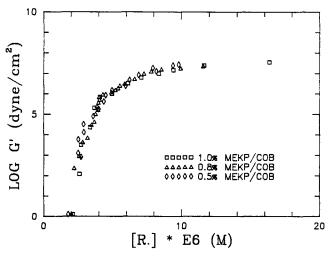
Figure 9 Shear storage modulus versus radical concentration for ST/UPE resin with MR = 4 cured at  $40^{\circ}C$
