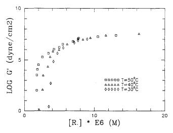
Figure 10 Shear storage modulus versus radical concentration for ST/UPE resin with MR = 4 and 1.0% MEKP/COB cured at various temperatures
