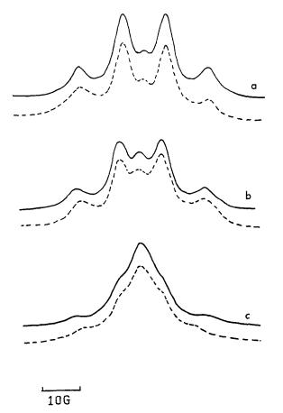
Figure 12 Comparison of simulated and experimental e.s.r. absorption spectra of ST/UPE resin with MR=2 and 1.0% MEKP/COB cured at 40°C:——, simulated spectra assuming (a) 20%, (b) 40%, (c) 80% UPE-end stable radical; ---, measured spectra at reaction times of (a) 100, (b) 760, (c) 1090s
